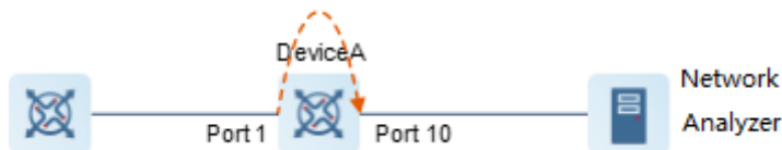
Figure 3-14 Operating Principle of Port Mirroring
